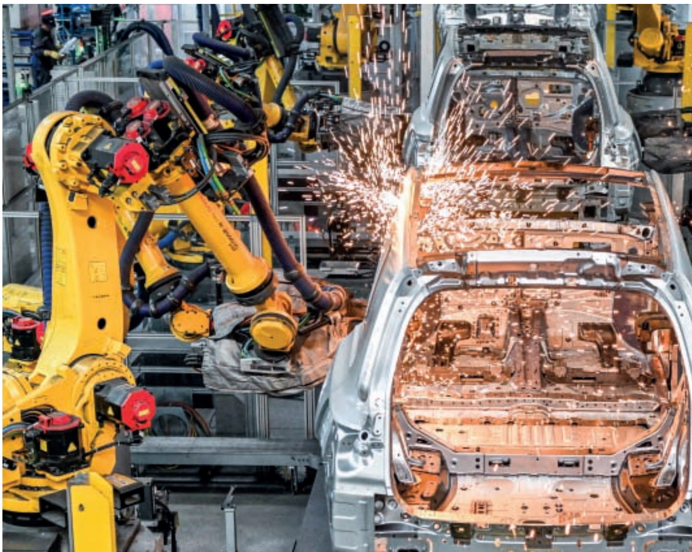
Robots weld bodysells of cars at a workshop of Chinese electric vehicle (EV) maker Li Auto Inc. in Changzhou, east China's Jiangsu Province, January 10, 2024. Ji Chunpeng
